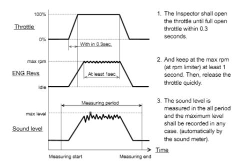
Sound limits: 114.0 dB/A before the race and 115.0 after the race. Exhaust pipes and silencers must fulfil all the requirements concerning sound control (please refer to the latest FIM Sound Regulations) available hereunder:
