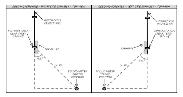
Silencers fitted with adapters aiming to reduce the sound level shall be permanently fitted. To make repetitive measurements, all motorcycles can be positioned into a small frame fixed on the ground, making sure to respect the 45° requirements. A squared frame helps the positioning of the motorcycle
