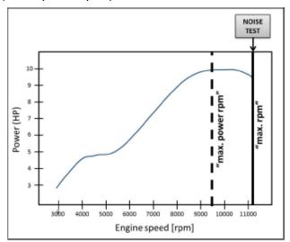
To conclude the test, the SCO releases the throttle quickly. The maximum noise value (dB/A) registered during the measurement interval is then read on the sound meter and recorded. This noise value shall not be rounded down to the nearest whole number.
